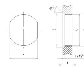
Installation direction: o-ring sits on chamfer.
